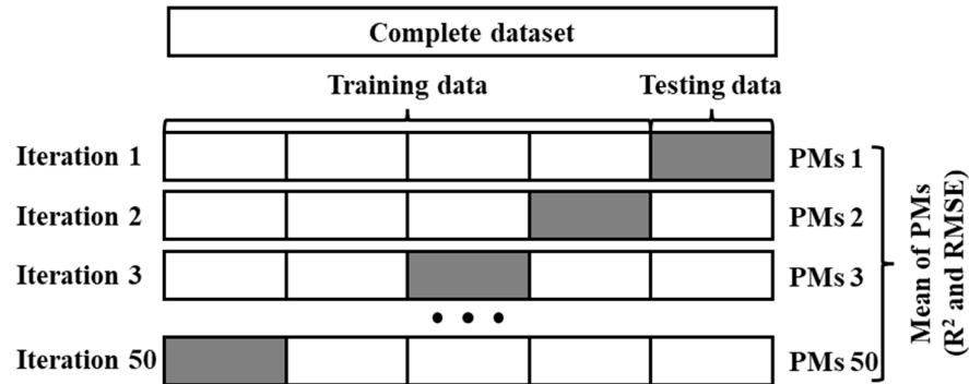
Figure 3. A schematic diagram of a 5-fold cross-validation method for computing the performance measures of different ML models. PMs: performance measures.
