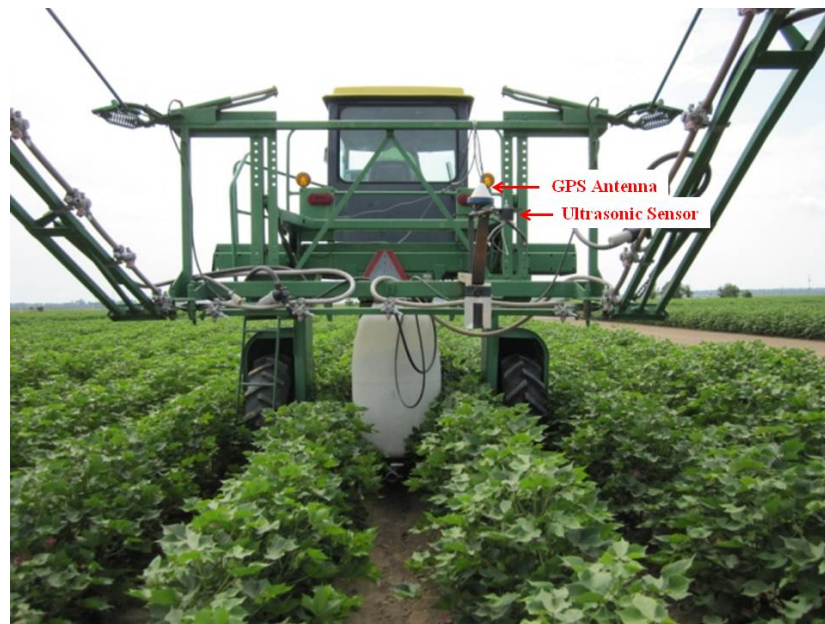
Figure 3. Ultrasonic plant height mapping system installed on a sprayer
