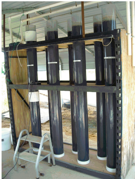
Figure 1 – Meso-scale lagoon column set-up supported with a metal rack. All sides of the metal rack were covered with plywood to maintain the liquid-sludge columns in the dark except for the topmost 0.3 m of each column, which was exposed to natural light.
