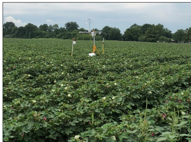
Figure 8. Eddy covariance system installed in a Mississippi cotton field to measure net ecosystem exchange of CO_2 and water from Anapalli et al. (2019).
