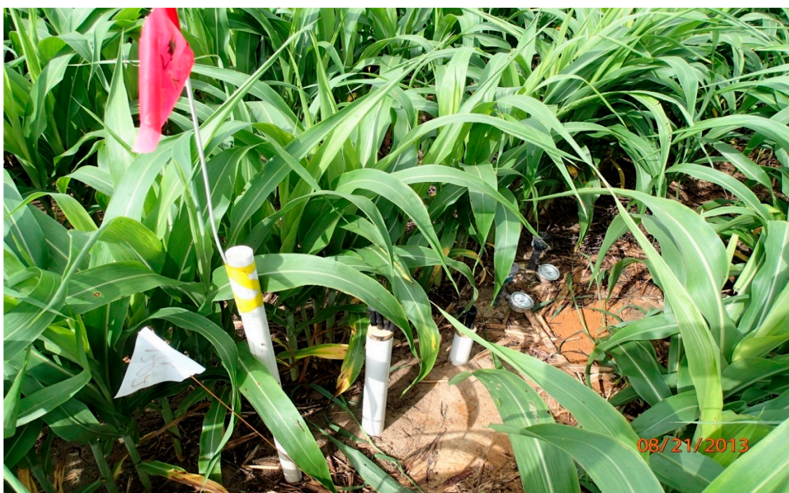
Figure 3. Installed suction lysimeters and soil moisture tensiometers.
