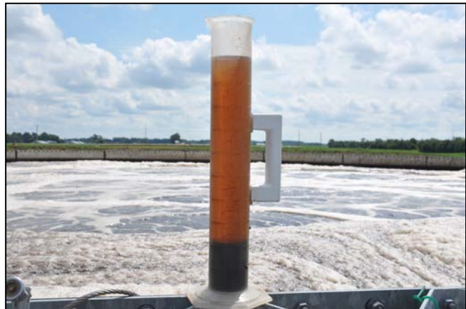
Start-up of the biological N removal unit with 1 liter of HPNS high performance nitrification sludge.
