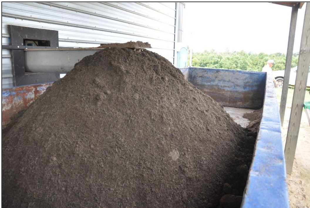
Separated manure solids being collected in a transportation bin.
