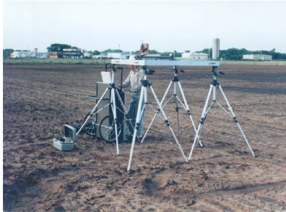
Figure IX-1. Photo of laser profilometer system including laser, position table, computer, controllers and power supply.
