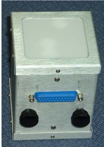
Figure 32. CROPSCAN Multispectral Radiometer (MSR). (Size is 8 X 8 X 10 cm).
