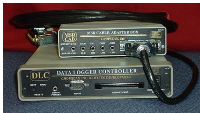
Figure 33. Data logger controller & cable adapter box.
