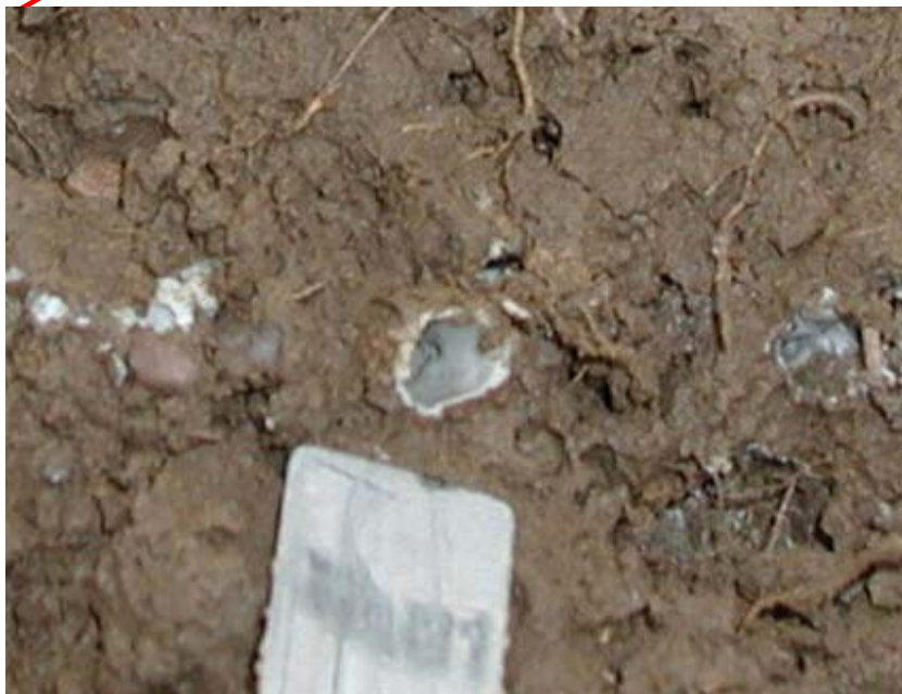
Figure 4. Lime slurry was surface applied to the lysimeters and rainfall added to highlight old root channels and earthworm burrows.
