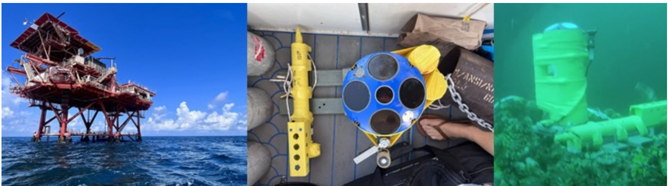
Figure 41. (left) South Pass 83 oil platform, (center) ADCP, CTD, and PAR sensors, (right) sensors in place on South Pass 83.
