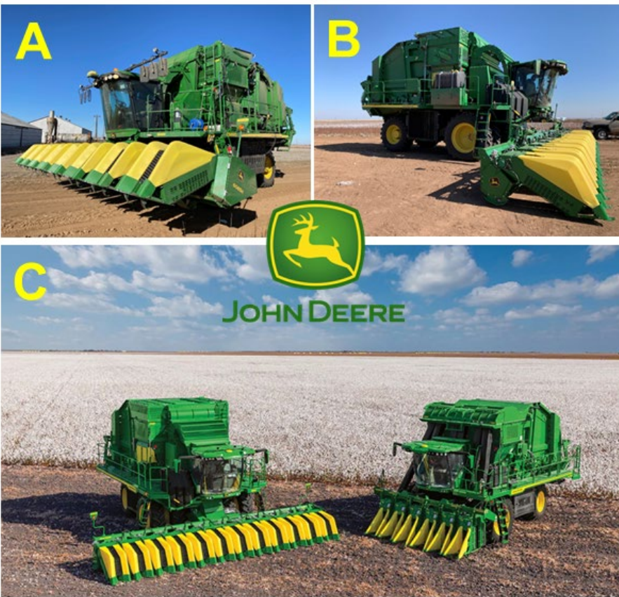
Figure 20. Work with John Deere on developing and evaluating the performance of a new field cleaner for stripper harvesters that increased material processing capacity by 25 percent, cleaning efficiency by 20 percent, and increased the value of cotton over $5 per bale resulting in $35 to $50 million of annual revenue increase for farmers. A) JD CS690 cotton stripper harvester previously built that uses the old 2 drum 60” wide cleaner design. B) JD CS770: Current state-of-the-art cotton stripper that uses the new 3 drum 75” wide cleaner design. C) Press photo of the new John Deere CS770 Cotton Stripper and CP770 Cotton Picker that help farmers harvest every pound of seed cotton possible while preserving cotton quality.
