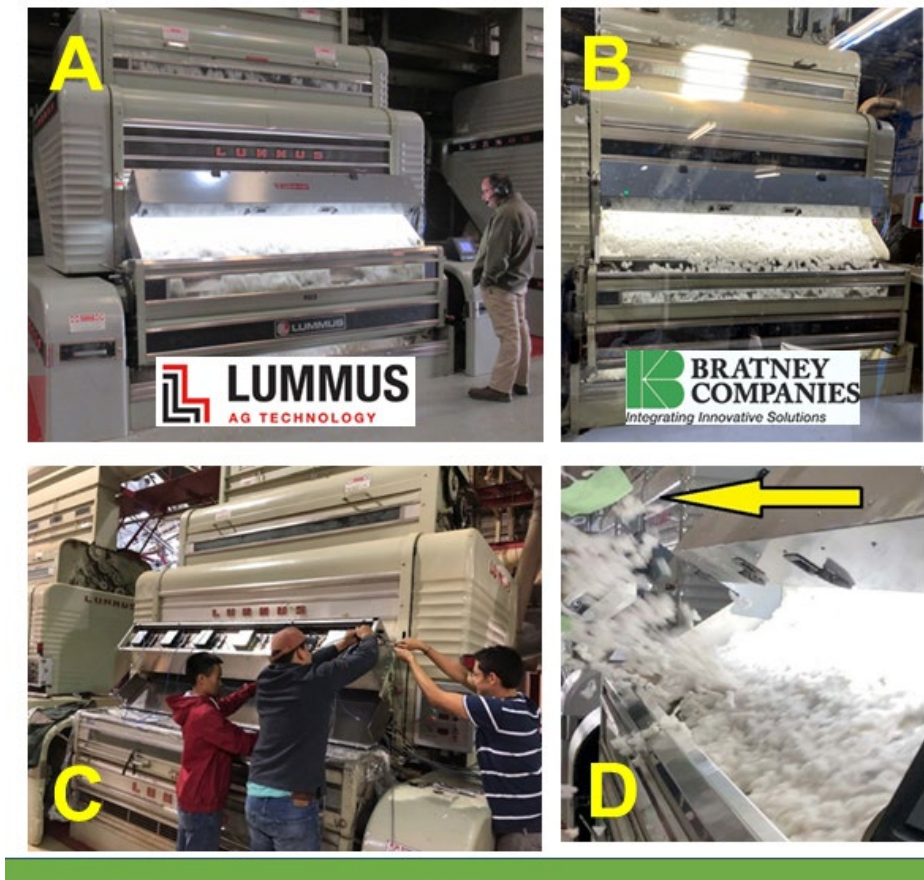
Figure 19. Technology developed by ARS and now commercially produced under the trade name “VIPR” detects and removes plastic and other contaminants from seed cotton before it enters the gin stand. Collaborative research and development agreements with Bratney Companies and Lummus Corporation led to VIPR™ Commercial Installation in Lummus Gins at A) Southeastern Gin, GA and B) Spade COOP Gin, TX. Lower images demonstrate C) technology is an ultra-low-cost, “bolt on” detection and removal system built using off-the-shelf parts that D) removes contaminants.
