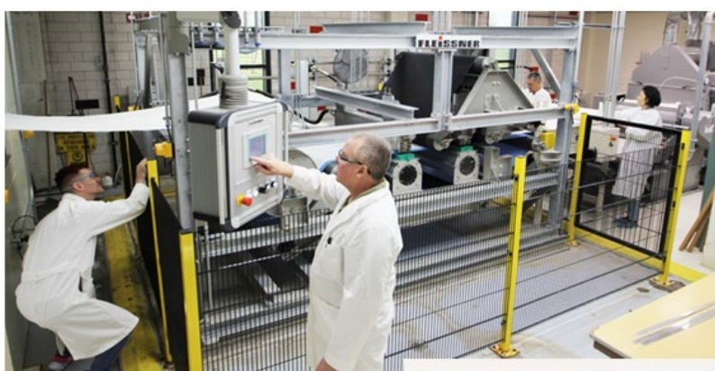
Figure 21. ARS researchers from left to right: Matthew Hillyer, Doug Hinchliffe, Pablo Salame, and Sunghyun Nam use the hydroentanglement process to fabricate nonwoven wipes in the nonwoven pilot plant at the Southern Regional Research Center in New Orleans. Cross-section of a cotton fiber with silver nanoparticles (black dots) synthesized in the primary cell wall. These silver nanoparticles have powerful antimicrobial properties, and these embedded nanoparticles kill bacteria on cotton after 50 washings.
