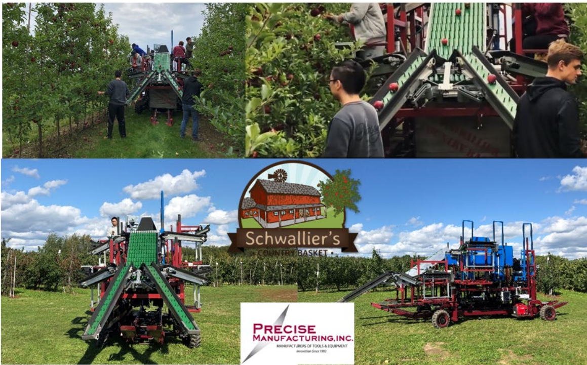
Figure 14. The new apple harvest assist and automated in-field sorting machine featuring a patented, automated fruit sorting system for grading and sorting apples into two quality grades (fresh market and cull or processing) at a speed of up to 12 fruits per second, an innovative bin filler design for automatically handling graded and sorted fruits, and automatic handling of empty and fully filled fruit bins or containers.
