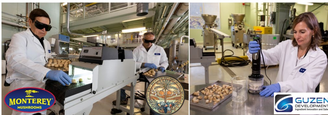
Figure 9. ARS researchers have developed an ultraviolet-B light treatment to transform mushroom-stalk waste into a vegetarian ingredient with a high level of vitamin D. When applied as a film coating to fruit bars and fresh-cut melons, the colorless, tasteless, edible powder helps preserve quality and safety and increases shelf life.
