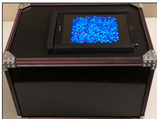
A low-cost, portable device for detecting and sorting Aflatoxin-contaminated corn kernels
