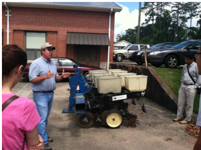
Research Agronomist Kip Balkcom points out residue management modifications made to a planter to improve success in establishing a crop in conservation systems.
