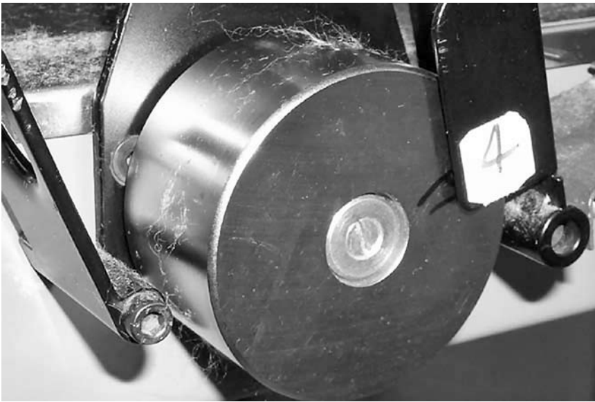
Figure 1. Sticky deposits on the draw frame creel drive rolls (Hequet and Abidi 2002).
