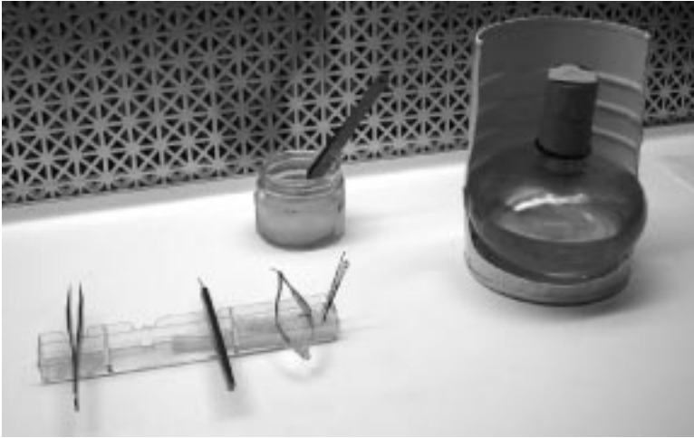
Fig. 1. Typical arrangement of equipment in the clean bench for dissections. The jar in the center contains ethanol and a small layer of cotton in the bottom. The dissecting tools are placed in the jar for at least 5 min, after which the alcohol is ignited by passing the tip over the alcohol lamp's flame ( see Note 9 ). They can then be positioned on a small tray (in this case, it was fashioned from the container in which the microscalpel was purchased) until needed for the dissection.
