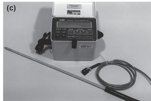
Fig. 7. Examples of various four-electrode probes: (a) burial probe, (b) insertion probe, and (c) bedding probe.
