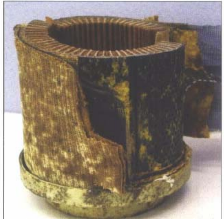
Leopard spots on the filter surface is a clear sign of microbiological growth
