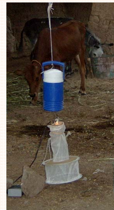
CDC light traps baited with CO2
