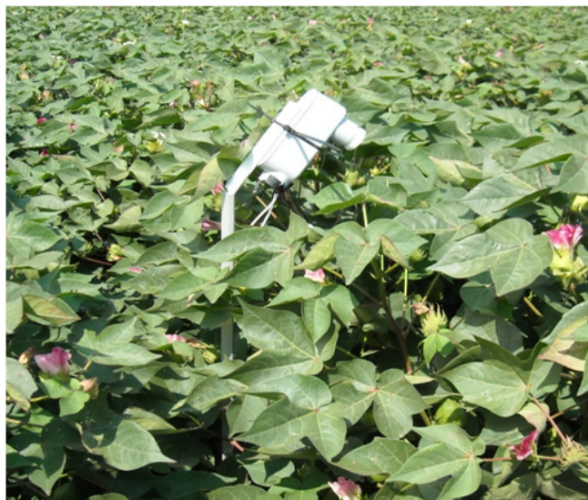
Figure 3. Infrared thermometer measuring cotton plant canopy temperature
