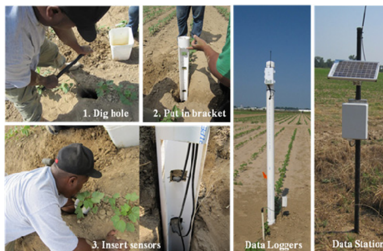
Figure 2. Installation of soil moisture sensors, data loggers, and the data station
