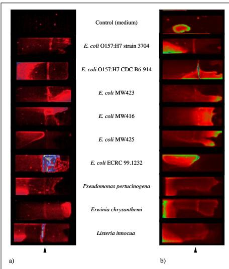
Figure 4. Fluorescence ratio images (a: 444/588 nm, b: 473/645 nm) of biofilm formations on stainless steel coupons in M9C (a) and TSB (b) media acquired with the portable hyperspectral imaging system. Coupons were submerged in 50-ml tubes containing 15 ml of medium for a 1-week at 37°C. The arrowheads indicate the medium fill lines.
